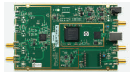
2. Model USRP B200 is an SDR/CR with one receive and one transmit channel on a single PCB powered by USB connection. Diligent
